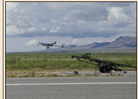
A Shadow UAV is launched from Condron Field in support of a network exercise at White Sands Missile Range. The Shadow is equipped with various camera systems to provide tactical intelligence, and a set of radios to help extend the wireless network's range in rough terrain.
